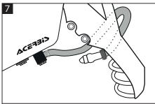
Attach the HUSQVARNA fuel line to the Acerbis tank (A) as indicated in the diagram.
