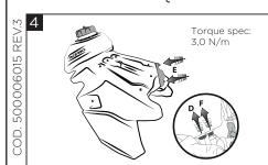
Assemble the pump (E) and the fasteners (D/F) on the Acerbis fuel tank.
