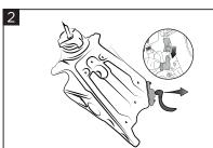
Disconnect the fuel pump cover cable and the fuel connector as indicated in the diagram. Remove the original tank. Sconnettere il cavo alimentazione della pompa. Scollegare connettore benzina.
